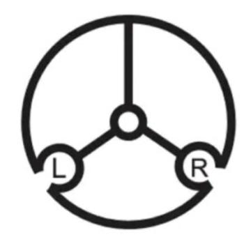
Half of all corner pillars shall have the shelf bracket(s) mounted to the left (L) slot and the other half to the right (R) slot.
